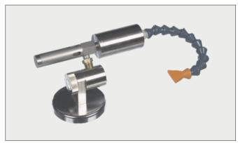
The Mini Spot Cooler utilizes a vortex tube to create one hot stream and one cold stream (see page 9). The cold air produced at the cold end is directed to the surface to be cooled using a flexible hose.
